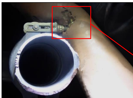
Photo No. 5: Coupling securing main portion of fractured spacer to the manifold partially embedded in flexible section of main fuel feed line
