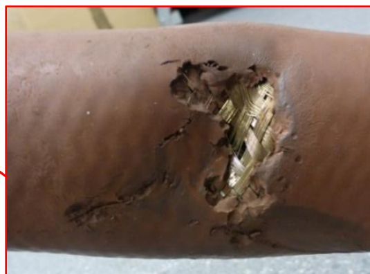
Photo No. 6: Damage to flexible section of main fuel feed line
