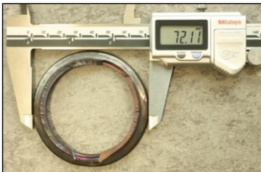
Photo No. 7: Maximum diameter of fractured spacer flange (72.11 mm)
