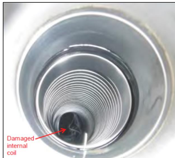
Photo No. 16: Damage to interior of flexible section of No. 2 engine's main fuel feed line
