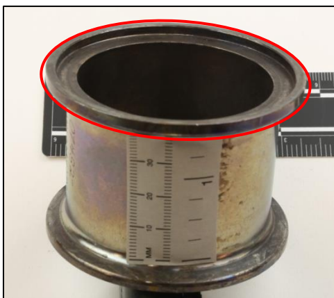
Photo No. 1: Recessed flange on engine side of spacer (circled)
