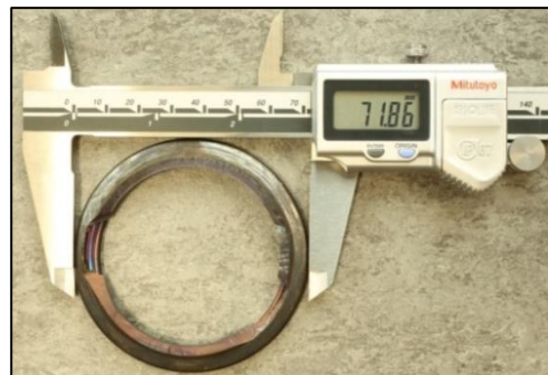
Photo No. 8: Minimum diameter of fractured spacer flange (71.86 mm)
