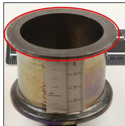
Photo No. 2: Non-recessed flange on manifold side of spacer (circled)
