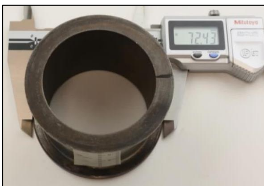
Photo No. 9: Maximum diameter of exemplar spacer flange (72.43 mm)
